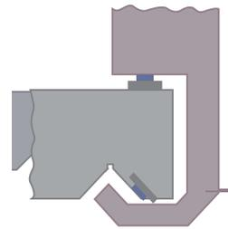
Integral dovetail guideway on Y axis enhances the performance.
