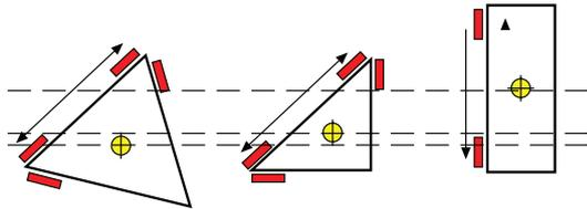
Patented TRICISION® bridge design with wider bearing separation, a lower centre of gravity and lighter weight than a conventional bridge coordinate measuring machine (CMM) beam.
