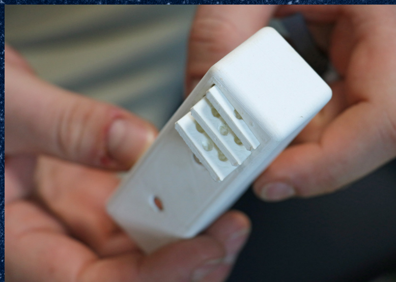
Using a 3D printer, toolcraft created this fixture, which can hold all 32 cerumen filters of a batch via three drawers.
