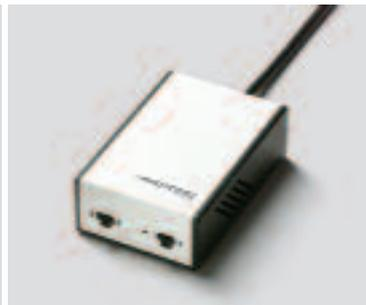
The **control unit** supplies the ringlight with a high frequent current (25 kHz) which is responsible for the flicker-free and homogen light of the fluorescence ringlight. The system operates vibration- and noiseless and can be supplied also with battery or akku. It contains the on/off-switch, the two-step brightness control and an ESD-socket.
