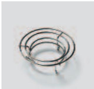
The **protection grating** is an optional feature of the Photonic fluorescence light to prevent that the user comes in touch with the fluorescence lamp by mistake. A contact between user and lamp would cause unwanted anti-static problems, especially at an ESD-safe workstation. The metal-made fence is conductive-connected with the ESD-socket and is unique on the machine-vision illumination market.
