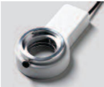
The **fluorescence ringlight** provides the illumination area with bright, uniform and homogen light. By a new smooth lamp ignition, a loss of lamp lifetime will be prevented. The housing is not thermal-conducting and made of anti-static material which causes the good ESD-qualities. The simple and gentle mounting-system is adaptable for objective-diameters up to 66 mm and can be fitted with custom-made adapters for special applications.
