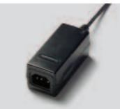
The switch-mode **power supply** has a voltage range of 100–240 V, 50/60 Hz and therefore can be used world-wide. It supplies the control unit with stable 24 V DC and frees the system from voltage variation.
