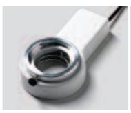
The **fluorescence ringlight** provides the illumination area with bright, uniform and homogen light. By a new smooth lamp ignition, a loss of lamp lifetime will be prevented. The housing is not thermal-conducting and made of anti-static material which causes the good ESD-qualities. The simple and gentle mounting-system is adaptable for objective-diameters up to 66 mm and can be fitted with custom-made adapters for special applications.
